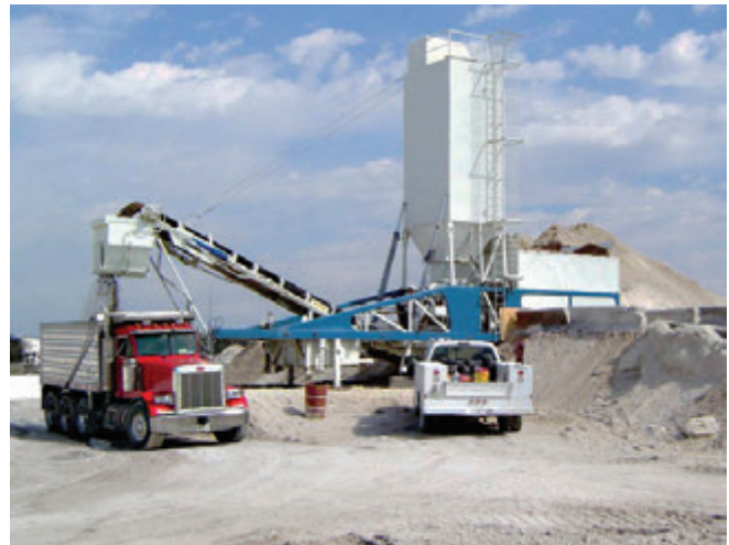
Figure 3.1. Mixing CTB in a continuous-flow-type pugmill.
